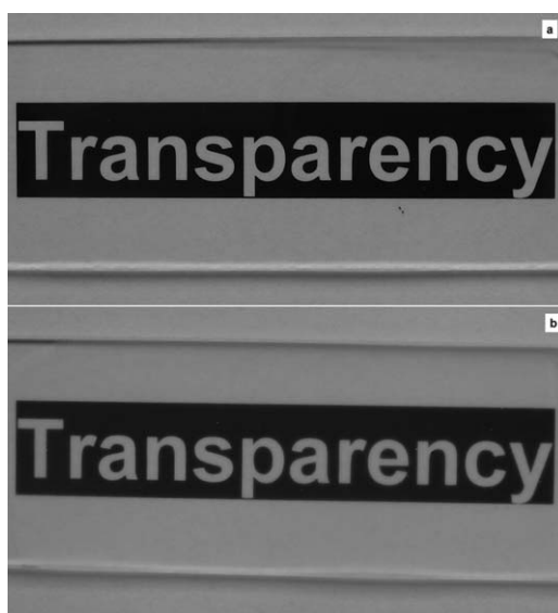
Figure 11. Nanocomposite films of (a) EVOH-MAOM-TMOS and NBt-MAOM-TMOS and (b) EVOH and NBt-MAOM-TMOS.
